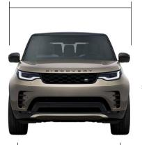
Front wheel track Air suspension 1,692.4mm
